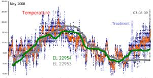
Above is a plot relating temperature to building movement as recorded by the electrolevels and the apparent - yet to be proven - benefit of applying the treatment. Sensor EL 22953 in particular appears to have stabilised.
