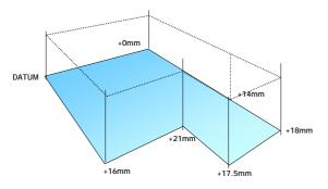
By the end of June 2009, moisture uptake by the tree has produced minor movement (also recorded by the electrolevels - see right) with the largest difference between stations of 1.1mm. See below.
